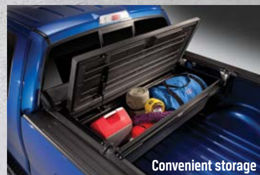
Elevated mounting for full bed floor access
